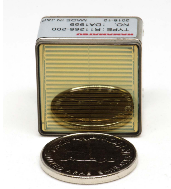
Figure 4: The Hamamatsu photomultiplier R11265U-200 used in the present work, next to one UAE Dirham coin.
