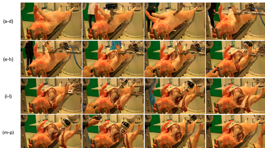
Figure 11. Stepwise shoulder removal using the MFC platform. The steps are ordered row by row, left to right. In brief, the steps show: (a) the entire carcass before cutting; (b) neck outer cut; (c) rib outer cut; (d) gripping; (e) chest outer cut; (f) bending #1; (g) inner cut #1; (h) bending #2 and inner cut #2. (i) bending #3; (j) inner cut #3; (k) inner cut #4; (l) bending #4; (m) inner cut #5; (n) inner cut #6; (o) inner cut #7, with removal completed; (p) shoulder removal complete. Note that the number of inner cuts and associated bends can vary from carcass to carcass, and as noted in Section 3.3, has been reduced as a result of developmental work. Image source: Alex Mason and Michaela Pincková, NMBU.
