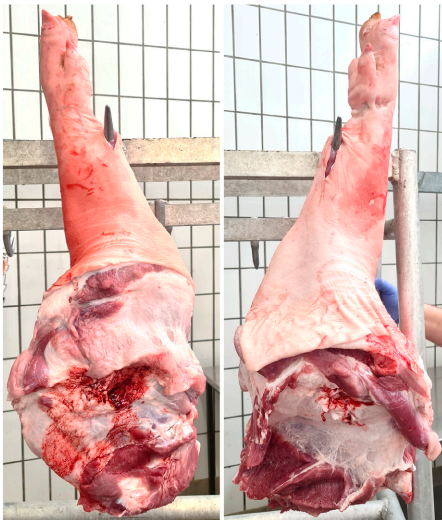
Figure 13. Example of shoulder removals performed by human (left) and robot (right). Image source, Alex Mason, NMBU.
