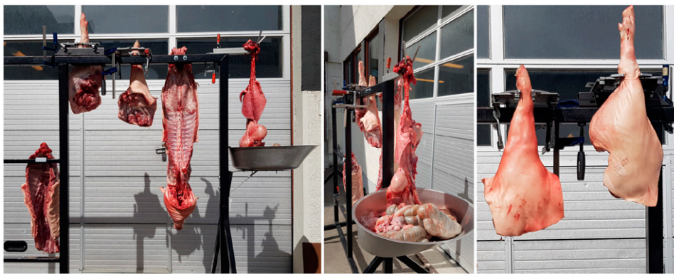
Figure 9. A prototype logistic unit, or rack, produced to hold the outputs of the MFC; those being hams, shoulders, the entire back with head, the entire belly and the complete organ set. The image on the left shows examples of all relevant parts affixed to the rack, while the centre and right images show fixation of the organ set and limbs, respectively. Images: Luis Eduardo Cordova-Lopez, NMBU.
