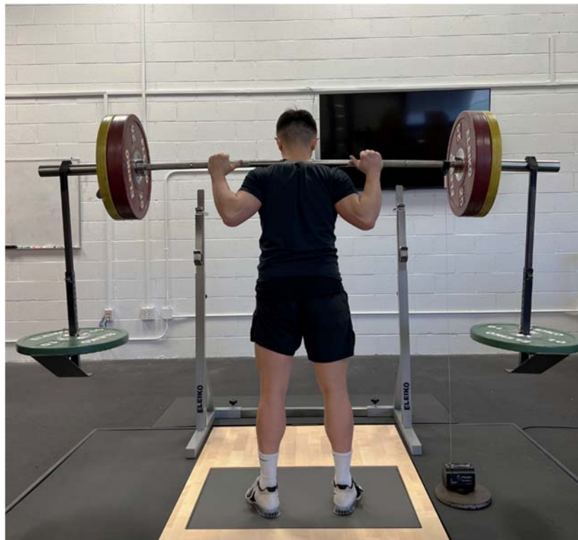
Figure 2. Force plate and linear position transducer set up during a back squat performed with accentuated eccentric loading.
