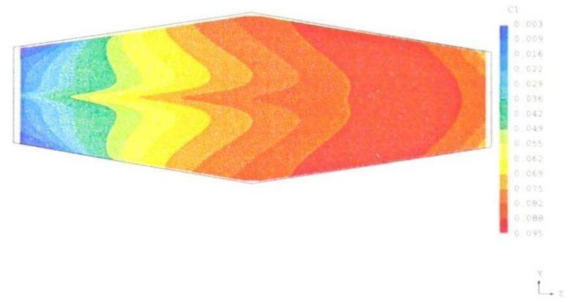
(b) Concentration Distribution Straight Jet Velocity 40m/s Length 6cm Time Step 0.4 Sec.
