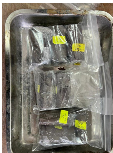
Fig. 1 Stabilized soil sample wrapped with plastic film for curing process
