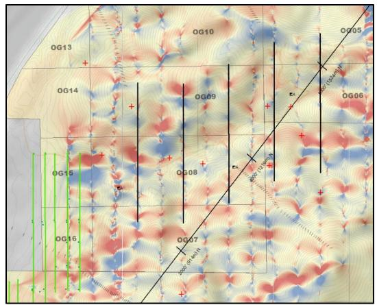
Figure 9.2. Area of proposed Osborne IP/ER survey. Five 1200' (360m) northsouth lines that cross the Osborne draw, each separated by ~400' (120m) are proposed. Green lines are of previously completed IP/ER survey. Black lines are proposed new lines.
