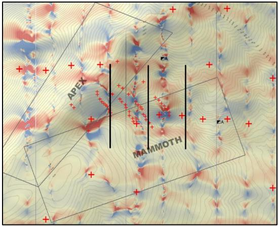
Figure 9.3. Area of proposed Mammoth IP/ER survey. Three 600' (180m) northsouth lines across the Mammoth gully, each separated by ~200' (60m), are proposed. Black lines are proposed new lines.
