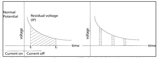
Figure 7.6. Time integrated measure of IP. On the left is a theoretical decay curve with voltage potential indicated by the hashed area. Because equipment cannot measure the continuous decay of voltage the curve is sampled at multiple points during discharge to reconstruct the decay curve, as shown on the right. Modified from Parasnis (1975).
