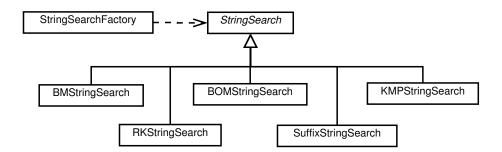
Figure 3.3: UML diagram of StringSearch class hierarchy.
