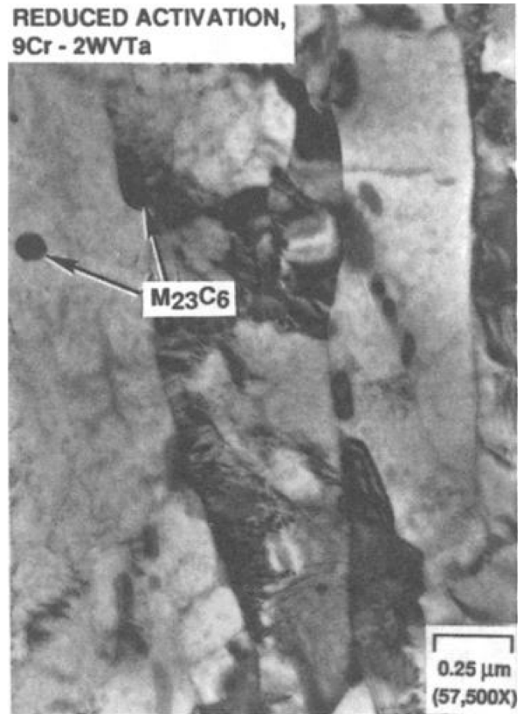
Figure 2.12: Bright field TEM images of a reduced-activation 9 Cr-2WVTa steel showing the grain structure and precipitate formation after tempering, from [3].
