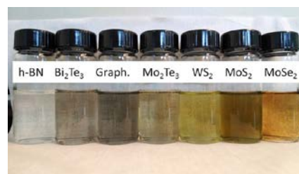
Figure 1: 2D nanoflakes suspended in a solution of isopropanol and deionized water.
