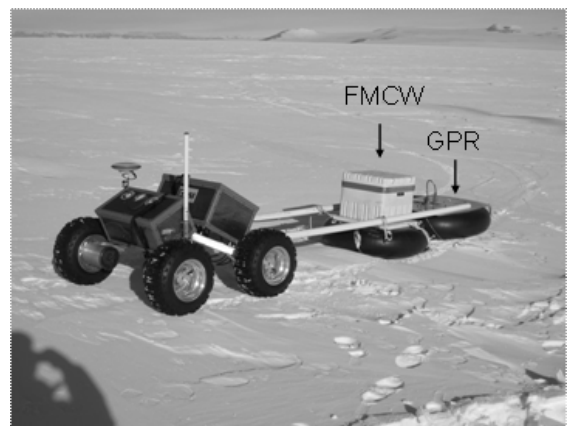
Figure 3. Yeti pulling a 2-10 GHz FMCW radar and a 400 MHz GPR antenna.
