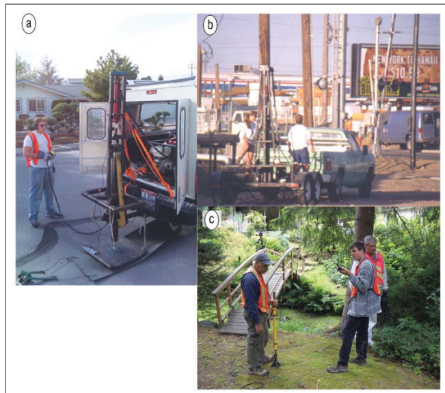
Figure 1. (a) Brady Flinchum operating the Boise State University hitch-mounted accelerated hammer source along a residential street in Reno, Nevada. A rubber mat is mounted below the plate to minimize road impact. (b) Trailer-mounted seismic source used to characterize groundwater aquifer through a high-traffic area in Boise, Idaho. (c) Portable slide hammer seismic source used to connect two weight drop seismic profiles along residential streets in Seattle, Washington.
