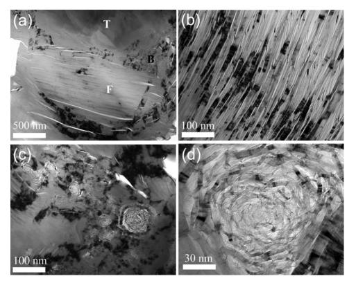
**Figure 4.** Bright-field TEM micrographs of NBG-18 grade graphite: (a) interface region constituting filler (marked F), binder (marked B), and turbostratic graphite (marked T), (b) filler particle at higher magnification, (c) binder region, and (d) rosette (QI particle) at high magnification.
