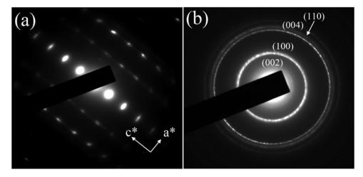
Figure 3. SAED diffraction patterns recorded from (a) filler particle and (b) rosette in the binder region of IG-110 graphite.
