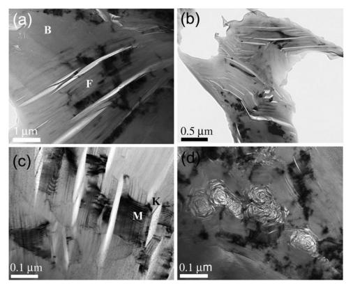
**Figure 2.** Bright-field TEM micrographs of IG-110 grade graphite: (**a**) interface region between a filler particle (marked F) and binder (marked B), (**b**) filler particle at high magnification, (**c**) filler particle with kink boundaries (marked K) and moiré fringes (marked M), and (**d**) binder region.
