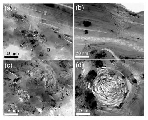
**Figure 6.** Bright-field TEM micrographs of PCEA grade graphite: (**a**) interface region constituting filler (marked F) and binder phase (marked B), (**b**) filler particle with cracks filled with porous amorphous carbon, (**c**) binder region, and (**d**) a rosette at high magnification.
