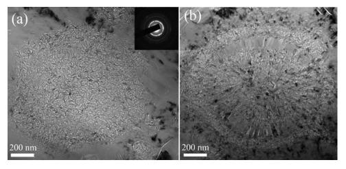
**Figure 5.** Bright-field TEM micrographs of spherical chaotic structures in NBG-18 grade graphite. Inset in (**a**) shows a typical SAED pattern recorded from these structures.
