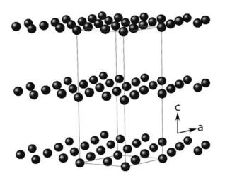
**Figure 1.** Schematic showing the layered crystal structure of graphite along with the unit cell outline.
