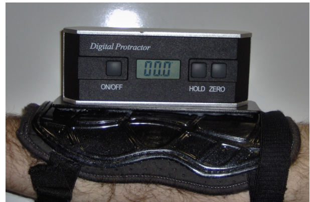
Figure 1. Modified digital inclinometer
