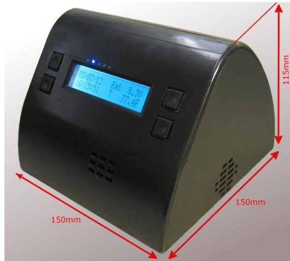
Figure 2. In-Home Air Quality Monitor. The monitor measures 150x150x115 mm and weighs 700g.
