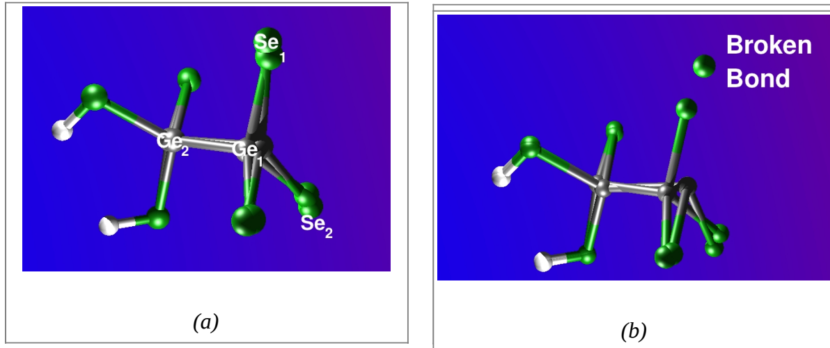
Figure 3: Overlaid atoms from the neutral and -1 charge state (a) and from the neutral and -2 charge state (b) showing principal distortions for self-trapping.
