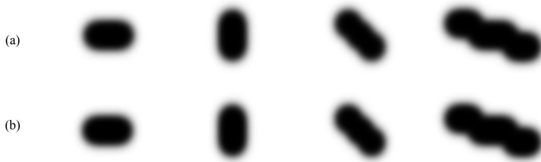
Figure 7: (a) Average images and (b) theoretical coverage for a three horizontal pixel, three pixels with vertical alignment, three pixels in 45 degree diagonal and a 20 degree line. resembles toner images when viewed with a microscope, and matches simulations of images created with these statistical properties.
