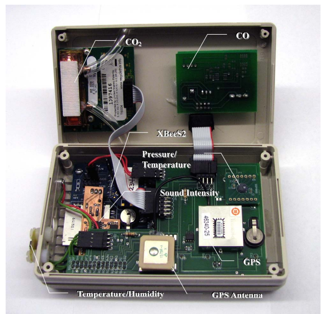
Fig. 5. The sensor module's internal layout. This configuration has carbon dioxide, carbon monoxide, temperature, humidity, barometric pressure, sound intensity, and GPS sensors.
