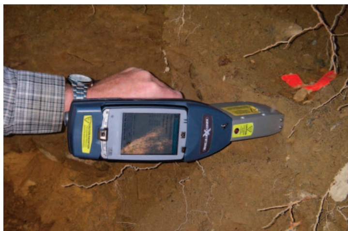
FIGURE 1 Example of a pXRF instrument being used to investigate the chemical composition of a soil profile. The quantitative results are reported on the instrument’s display. IMAGE COURTESY OF GWENDY HALL, GEOLOGICAL SURVEY OF CANADA
