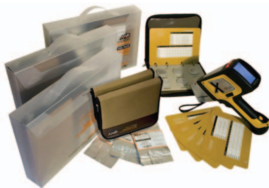
FIGURE 4 An example of a suite of reference materials for field calibration of pXRF devices. Each packet contains six plastic wells, each of which contains a pressed powder disk made from a certified reference material; each disk is covered by a thin foil to make it suitable for rugged field conditions. IMAGE COURTESY OF MIKE MCWHIA, AFRICAN MINERAL STANDARDS
