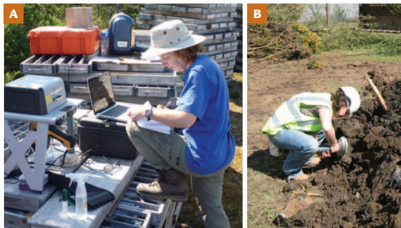
FIGURE 2 (A) Portable XRF instrument mounted under a table for on-site chemical analysis of drill core samples. IMAGE COURTESY OF GWENDY HALL (B) Handheld device being used to survey soil contamination at a former industrial site. IMAGE COURTESY OF M. H. RAMSEY, UNIVERSITY OF SUSSEX
