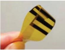
Figure 9. Ink-jet printed thermoelectric device on Kapton [54]
