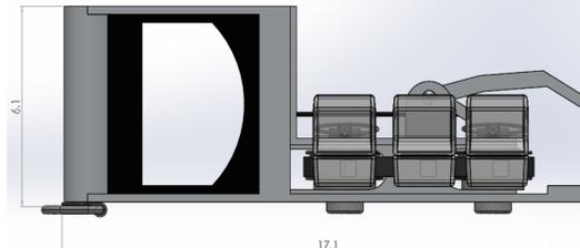
The claw is gone in favor of a u-channel mounted to the top of the clamshells. When the trigger is squeezed, a rod on top of the device is pulled back, and the clamshell opens. To close the clamshell, the trigger is released and the springs in the trigger push the rod and in turn the lid back forward. The rod hits the clamshell and it snaps close using the springs in the lid.
