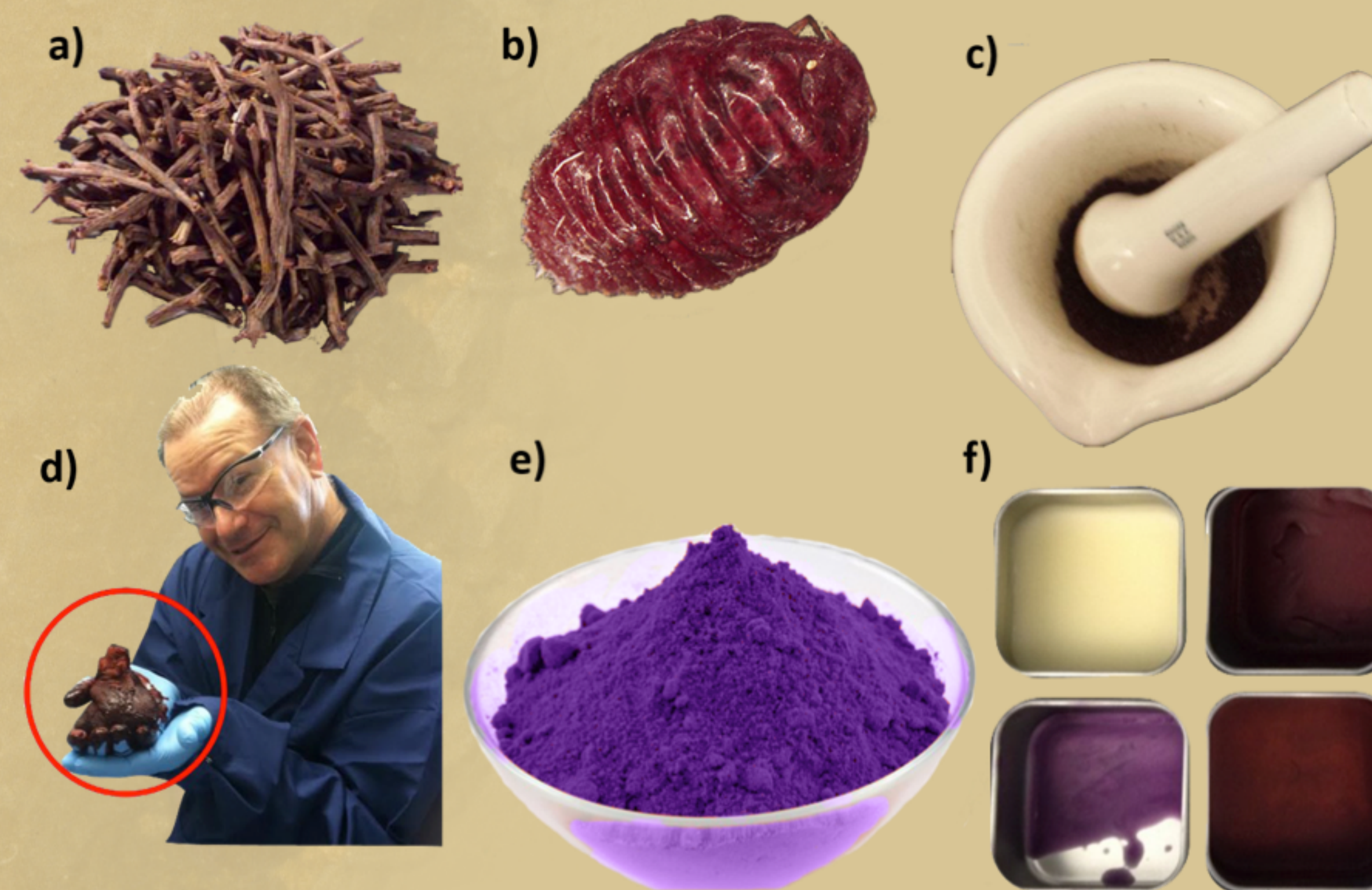
Figure 1: Raw (a) madder root and (b) Kermes\Cocheinal. Raw materials were (c) ground into a powder via mortar and pestle then allowed to steep in a water bath for 24-72 hours to release the pigments into solution. (d) The larger pieces of material were filtered from the solution using a cheesecloth, removed, and discarded. To the pigment solution, mordants, metal salts, and/or alkali salts were added to induce color change. The solvent was then evaporated off and (e) the resulting product was crushed into a fine powder and (f) subsequently set into a wax binder and placed into a metal tin.
