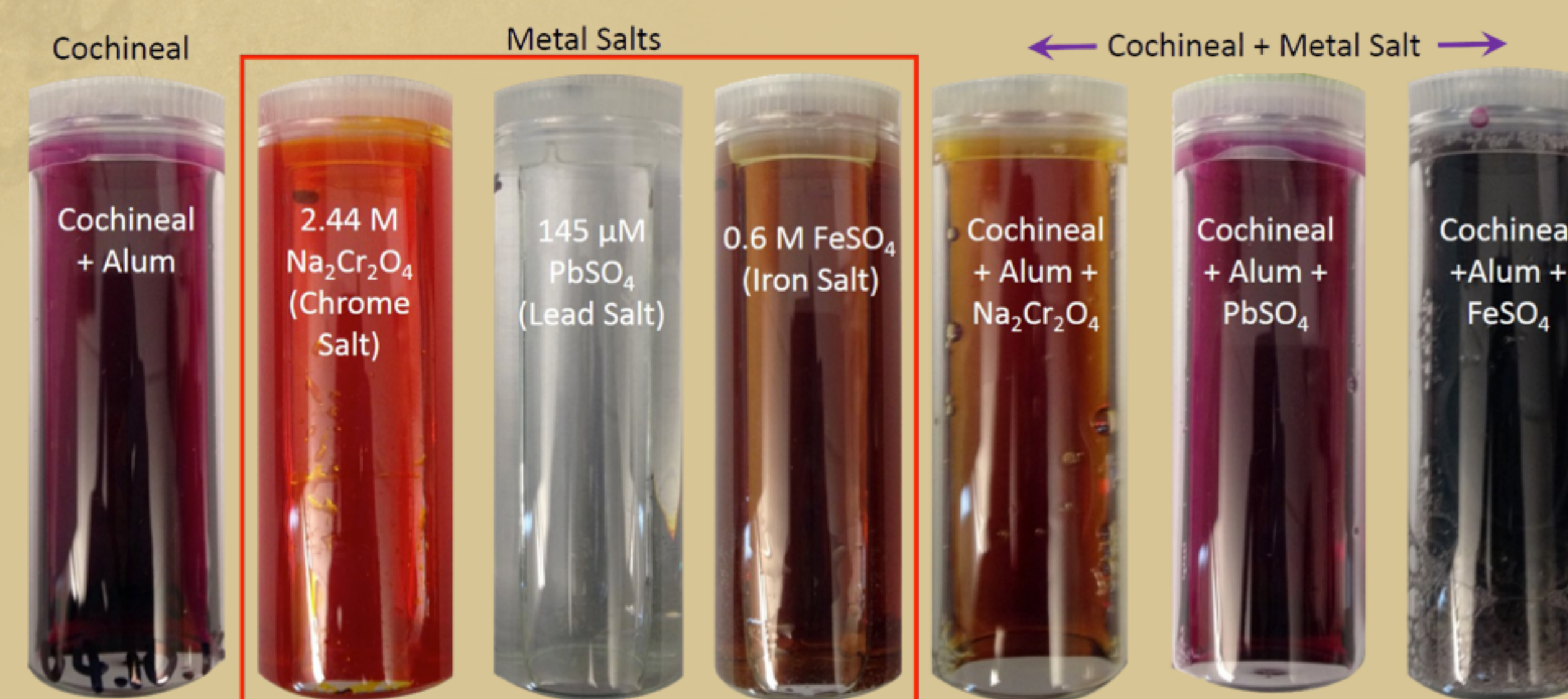
Figure 2: Image illustrating the effect of mixing metal salts (100 μL of 2.4 M chrome (Cr), 300 μL of 145 μM lead (Pb), and 100 μL of 0.6 M iron (Fe)) with a cocheinal and alum solution.
