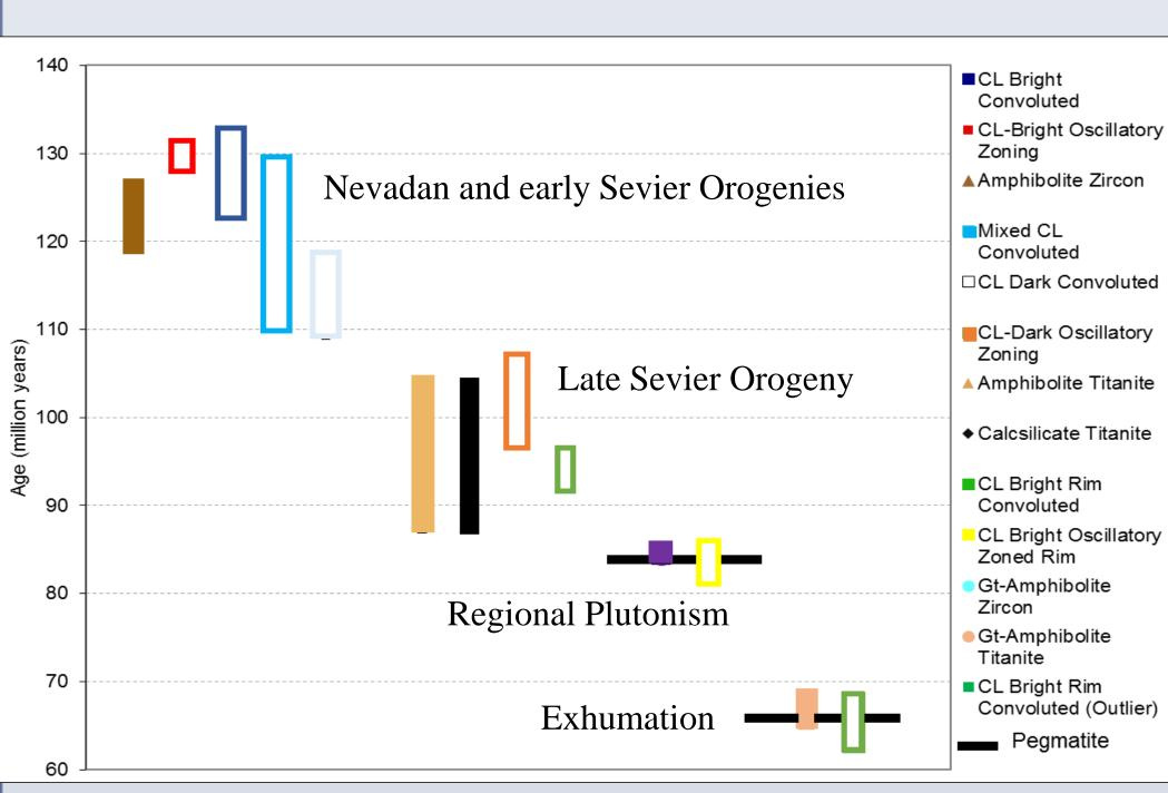
Figure 6. The zircon LA-ICPMS age data of this study (hollow) as compared to literature on rocks from the surrounding units (solid). (Alexander, 2007; Dye, unpublished)
