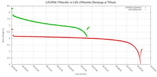
Figure 9.1 LiFePO4 vs LiPo - Discharge Data
