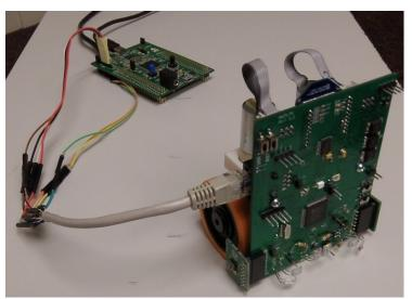
Figure 7.5 Robot with Programmer/Serial Port
