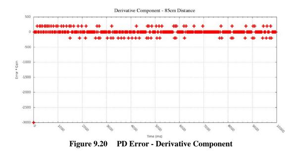
Combining both of these components into the total error allows this sum to be used for error correction as the robot navigates the corridor. The pulse width modulation controller uses this error value and proportionally adjusts the speed of each motor (positively or negatively), which results in a stable system. This data is not intended to show success of the controller but instead to show the successful integration of all components.
