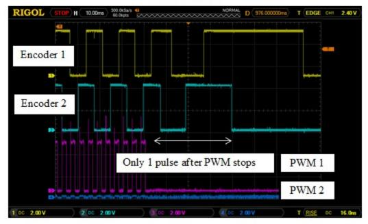
b) Motor brake Figure 6.6 H-Bridge Stop vs Brake
