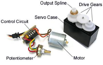
Figure 4.3 Servo Motor Breakdown
