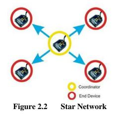
Many chipsets are available that implement the ZigBee protocol. The research in [14] has selected the MG2455 manufactured by Radio Pulse. Much like the well-known XBee module, the MG2455 is able to carry out mesh and star networking between embedded systems. Two robots carried out experiments to demonstrate the usefulness of ZigBee during collaboration.
