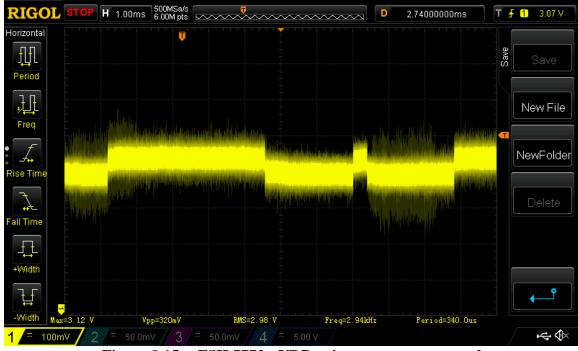
Figure 9.15 FSH 7773 - VDD using a common ground
