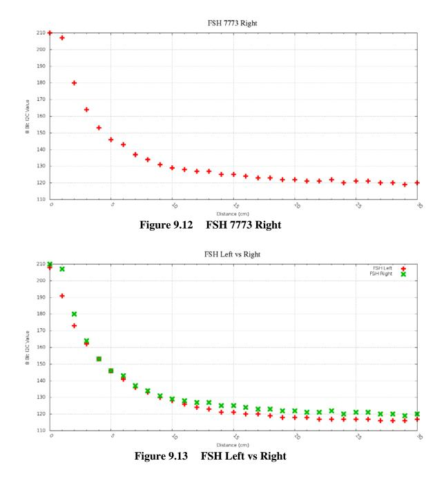
The noise test for the FSH 7773 shows a large amount of improvement over the previously analyzed proximity circuit. While there is only 8 bits of resolution with the FSH 7773, the data is much less noisy. Figure 9.14 shows that there are only 2 units of change out of 256 units of resolution equating to 0.7% error.
