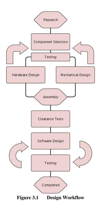
After several phases of component selection, testing, and design, a final assembly will emerge. Testing can then begin to ensure that all aspects of the mechanical design combine together as required without problems such as wheel rub, screw alignment, and ground clearance.
