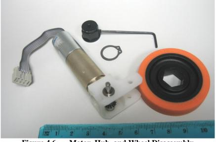
Figure 4.6 Motor, Hub, and Wheel Disassembly
