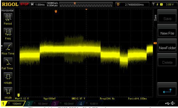
Figure 9.16 FSH 7773 - V\_LED using a common ground
