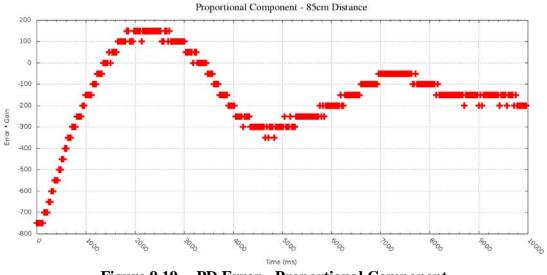
Figure 9.19 PD Error - Proportional Component
