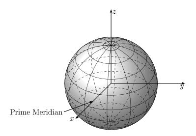
Figure 2.6: An illustration of the ECEF coordinate system.
