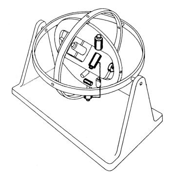
Figure 2.1: A simplified drawing of the ship's inertial navigation system[15].
