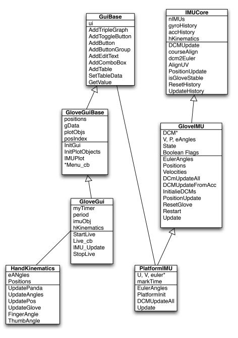
Figure 4.17: GloveGui UML Diagram
