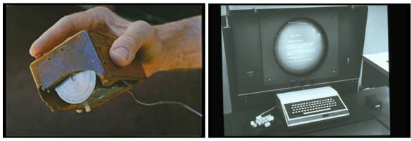
(a) First Mouse[12](b) First Mouse and Screen[4]Figure 1.3: The First Computer Mouse and Screen
