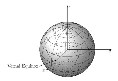
Figure 2.5: An illustration of the ECI coordinate system.
