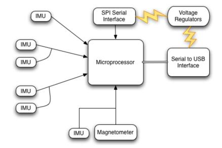
Figure 4.7: Block Diagram of GyroGlove Controller and IMU Boards
