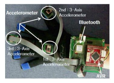
Figure 1.12: KHU-1 Korean Accelerometer Glove[23]
