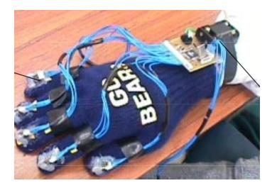
Figure 1.9: Acceleration Sensing Glove[24]
