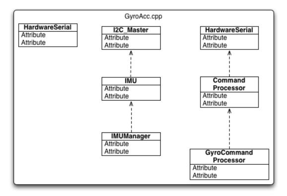
Figure 4.8: GyroGlove Firmware Architecture Block Diagram
