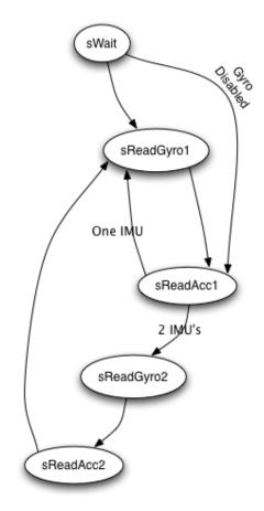
Figure 4.13: Partial State Machine Diagram for the IMU Class
