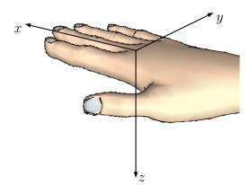
Figure 1.14: Body Reference Frame for Finger
