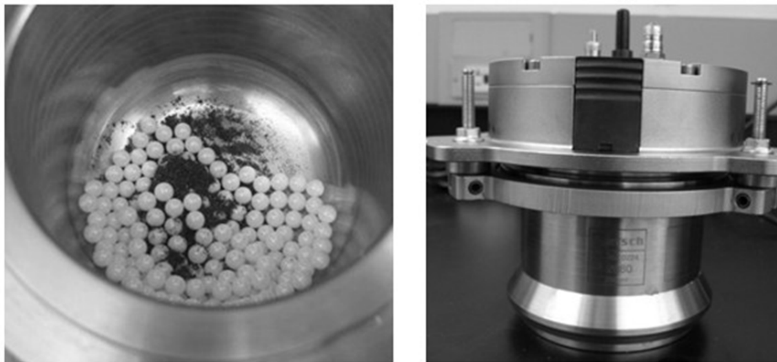
Figure A.3 Images of the 250 mL milling vessel loaded (a) with YSZ media and dysprosium filings in a 14:1 mass ratio with a total dysprosium mass of 5 grams and (b) after sealing with a lid consisting of gas purging and in situ temperature and pressure measuring capabilities. The in situ measuring capabilities allowed for a kinetics study on the nitridation reaction in the formation of DyN.
