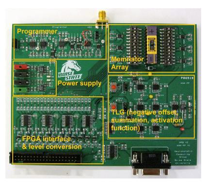
Figure 4.11: PCB built for this project consisting of programming circuit, memristor array, and ANN
