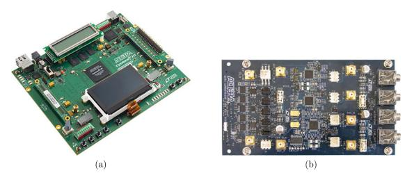
Figure 3.12: FPGA development board and DSP board
