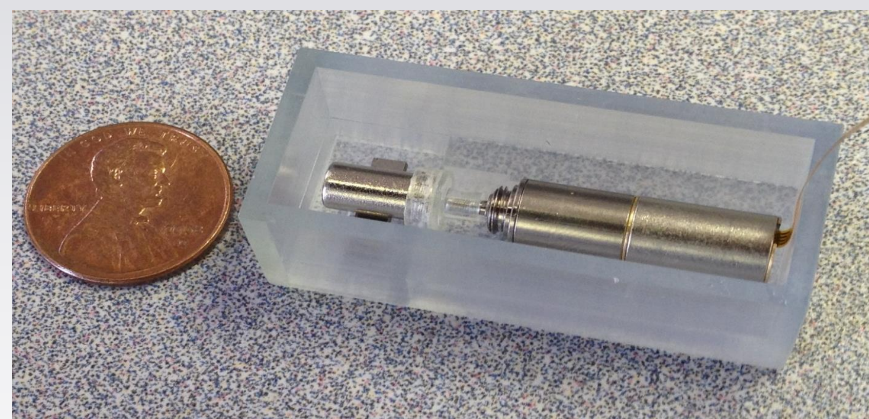
Previous prototype moving liquid from right to left over a rotating magnet K. Ullakko, L. Wendell, A. Smith, P. Mullner, G. Hampikian, Smart. Mater. Struct. 21 (2012) 115020
