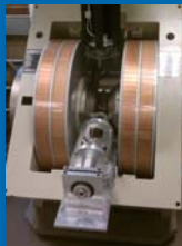
Figure 1: Vibrating Sample Magnetometer (VSM) with electromagnet and rotation apparatus (OMMD) inserted between the pole pieces. The motor and camera used to take images is missing in this image.
