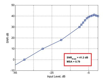
Figure 7.31: Simulated SNR vs input sinewave amplitude for the second-order KD1S modulator.
