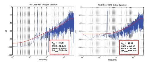
**Figure 4.12:** Simulated NTFs for the first-order KD1S modulator with the op-amp open-loop gain ( $A_{OL}$ ) of 50 dB and 25 dB. Again here,  $f_{s,new} = 800$  MHz,  $f_{un} = \frac{3}{8}f_{s,new} = 300$  MHz,  $K_{path} = 8$ , OSR = 8, and BW = 6.25 MHz.
