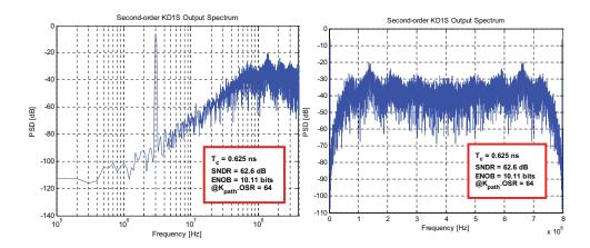
**Figure 5.12:** Spectre simulated PSD (log and linear frequency scales) of the secondorder KD1S modulator with comparator delay  $T_c = 625$  ps and the first comparator is clocked on  $\phi_{2-1}$ . Here,  $f_s = 100$  MHz,  $K_{path} = 8$ ,  $f_{s,new} =$ 800 MHz,  $f_{un} = \frac{3}{8}f_{s,new} = 300$  MHz, OSR = 8, and BW = 6.25 MHz.
