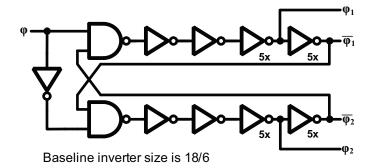
**Figure 7.8:** The non-overlapping clock generator for generating phases  $\phi_1[i]$ ,  $\overline{\phi_1[i]}$ ,  $\phi_2[i]$  and  $\overline{\phi_2[i]}$  from the DLL outputs  $\phi[i]$ , where i = 0, 1, ...7.
