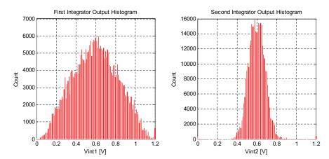
first integrator has excursions beyond 60% of  $V_{DD}$  due to excess delay in the comparator.
