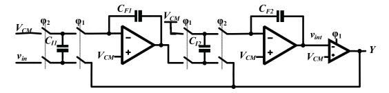
Figure 3.7: A switched-capacitor implementation of the second-order DSM.
