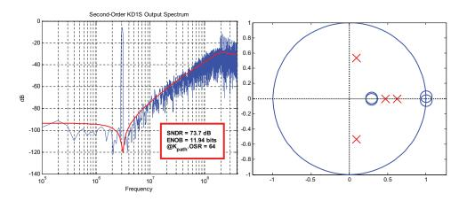
**Figure 6.15:** Simulated PSD of the output and the NTF pole-zero plot for the secondorder CIFB-type KD1S modulator. Here,  $f_s = 100$  MHz,  $K_{path} = 8$ ,  $f_{s,new} = 800$  MHz, OSR = 8, and BW = 6.25 MHz.
