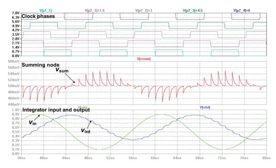
**Figure 4.5:** Transient simulation of a *K*-path integrator showing the integrator input and output, the op-amp summing node and the clock phases.
