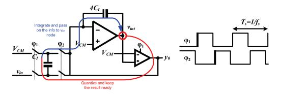
Figure 3.5: A first-order discrete-time delta-sigma modulator.
