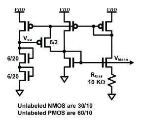
Figure 7.6: The self-biased reference (BMR) used in the DLL.
