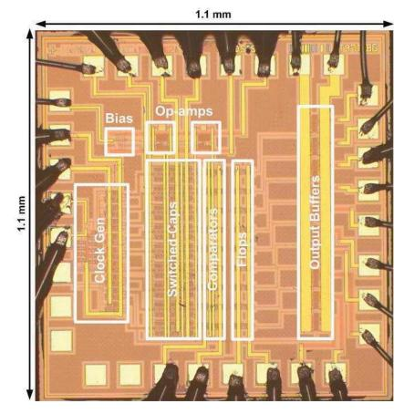
Figure 7.28: Die micrograph for a second-order KD1S test chip designed in 500-nm CMOS process.
