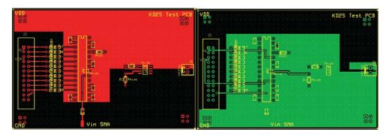
**Figure 7.37:** (a) Top layer (power plane) and (b) bottom layer (ground plane) of the test board.
