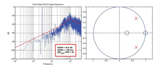
Figure 4.18: Matlab simulated PSD of the output and the NTF pole-zero plot for the first-order KD1S modulator with  $f_{s,new} = 800$  MHz,  $f_{un} = 300$  MHz,  $K_{path} = 8$ , OSR = 8, BW = 6.25, and the comparator delay  $T_c = T_s/K_{path} = 1.25$  ns.
