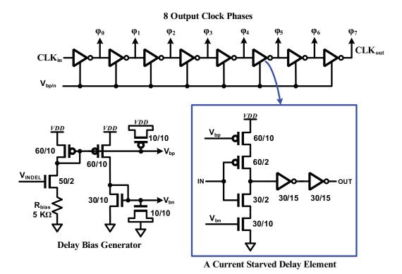
Figure 7.7: The voltage controlled delay-line (VCDL) with the delay bias generator used in the DLL.
