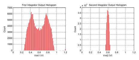
**Figure 5.5:** Histogram of the integrator states for the second-order KD1S modulator for the response seen in Figure 5.4.
