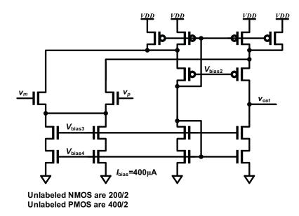
Figure 7.16: Single-ended op-amp employed in the first switched-capacitor integrator.
