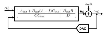
**Figure 6.12:** The equivalent ABCD matrix representation for a KD1S loop-filter after incorporating the integrator non-idealities.
