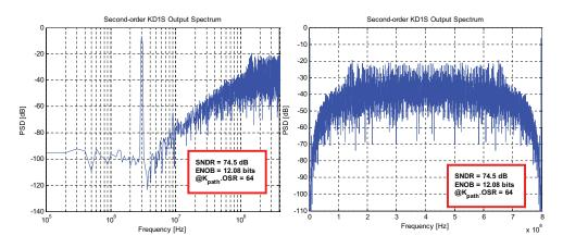
Figure 6.17: Spectre simulated spectrum for the second-order KD1S modulator implemented with switched-capacitors and  $f_{un}$  limited op-amp (log and linear frequency axes). Here,  $f_s = 100$  MHz,  $K_{path} = 8$ ,  $f_{s,new} = 800$  MHz, OSR = 8, and BW = 6.25 MHz.
