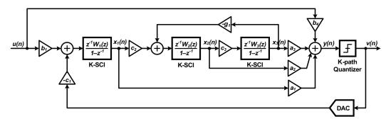
Figure 6.18: The synthesized third-order, single-bit CIFF KD1S modulator.
