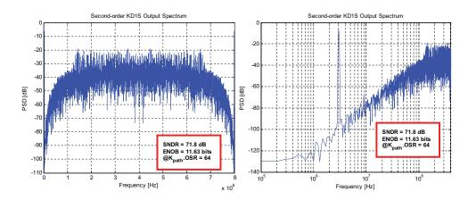
Figure 5.4: Spectre behavioral simulation result for the second-order KD1S modulator with ideal components. Here,  $f_s = 100$  MHz,  $K_{path} = 8$ ,  $f_{s,new} = 800$  MHz, OSR = 8, and BW = 6.25 MHz. The quantizer and op-amps are ideal.
