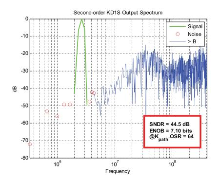
**Figure 7.32:** Simulation results for the second-order KD1S modulator designed in 500nm CMOS. IIn these results,  $f_{in} = 2.67$  MHz,  $f_s = 100$  MHz,  $K_{path} = 8$ ,  $f_{s,new} = 800$  MHz,  $K_{path} \cdot OSR = 64$ , and BW = 6.25 MHz.
