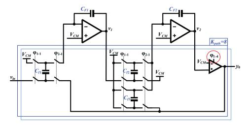
Figure 5.16: The second-order KD1S modulator with modified clock scheme to accommodate the  $T_c = T_s/K_{path}$  (or  $z^{-1}$ ) delay in the comparator.
