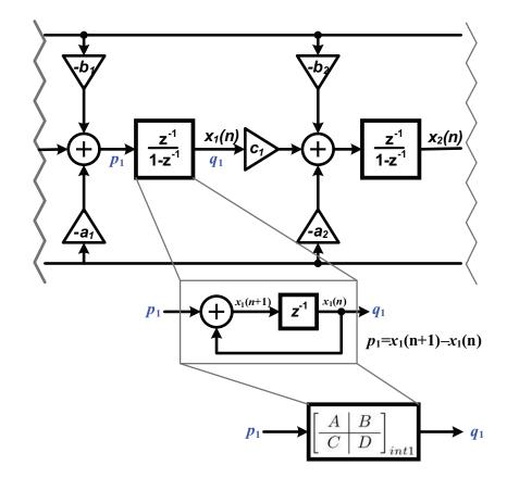
Figure 6.11: Illustration of the state-space embedding method for the non-ideal integrator.
