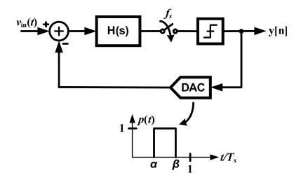
**Figure 3.17:** Block diagram of a continuous-time delta-sigma modulator. Here the feedback DAC pulse shape is shown as a generic rectangular pulse with excess loop delay ( $\alpha$ ), encountered in practical CT-DSM designs..
