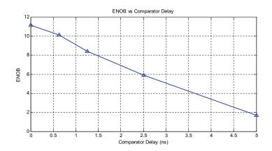
Figure 5.20: Effective resolution (ENOB) vs the Comparator delay for the secondorder KD1S modulator measured with sinusoidal inputs. Here, the effective clock frequency is  $f_{s,new} = 800$  MHz and BW = 6.25 MHz.
