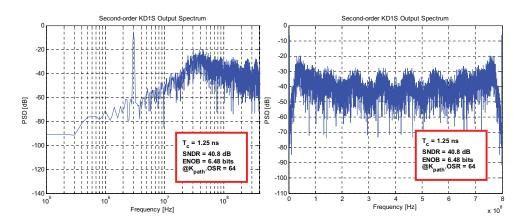
**Figure 5.14:** Spectre simulated PSD (log and linear frequency scales) of the secondorder KD1S modulator with comparator delay  $T_c = 1.25$ ns and the first comparator is clocked on  $\phi_{2-1}$ . Here,  $f_s = 100$  MHz,  $K_{path} = 8$ ,  $f_{s,new} = 800$  MHz,  $f_{un} = \frac{3}{8}f_{s,new} = 300$  MHz, OSR = 8, and BW = 6.25 MHz.
