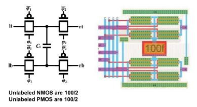
Figure 7.15: Switched-capacitor block with the corresponding layout.
