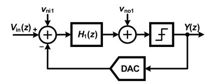
Figure 4.24: Noise sources in a first-order KD1S modulator.
