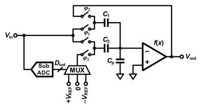
Figure 3.1: A 1.5-bit pipelined stage (MDAC) [1].
