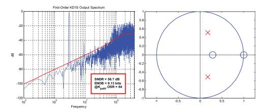
Figure 4.11: Simulated PSD of the output and the NTF pole-zero plot for the first-order KD1S modulator with  $f_{s,new} = 800$  MHz,  $f_{un} = \frac{3}{8}f_{s,new} = 300$  MHz,  $K_{path} = 8,OSR = 8$ , and BW = 6.25 MHz.
