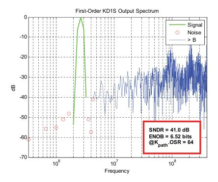
**Figure 7.30:** Simulation results for the first-order KD1S modulator designed in 500nm CMOS. In these results,  $f_{in} = 2.67$  MHz,  $f_s = 100$  MHz,  $K_{path} = 8$ ,  $f_{s,new} = 800$  MHz,  $K_{path} \cdot OSR = 64$ , and BW = 6.25 MHz.
