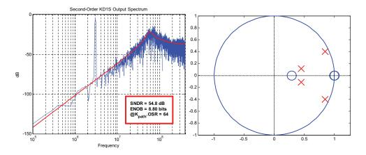
**Figure 5.19:** Matlab simulated PSD of the output and the NTF pole-zero plot for the second-order KD1S modulator with  $f_{s,new} = 800$  MHz,  $f_{un} = \frac{3}{8}f_{s,new}$ ,  $K_{path} = 8$ , OSR = 8, and  $T_c = 1.25$  ns (or  $z^{-1}$ ).
