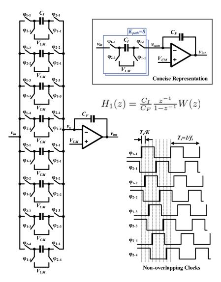
**Figure 4.2:** A *K*-path switched-capacitor integrator with a shared op-amp with the associated time-interleaved clocking scheme. A concise graphical representation for the *K*-SCI is shown in the inset.
