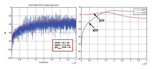
**Figure 4.10:** KD1S noise-shaping with an op-amp with finite unity gain frequency  $(f_{un} = \frac{3}{8}f_{s,new} = 300 MHz)$ . The second plot shows the NTF and STF for the modulator. Here,  $f_s = 100$  MHz,  $K_{path} = 8$ ,  $f_{s,new} = 800$  MHz, OSR = 8, and BW = 6.25 MHz.
