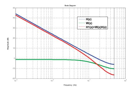
**Figure 4.4:** A plot showing the *K*-path integrator magnitude response for  $f_{un} = 1.5 f_s$ . Here, H(z) is the near-ideal integrator response, W(z) is the response of the charge spreading filter and  $H_1(z) = W(z)H(z)$  is the response of the *K*-path integrator.
