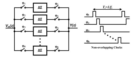
Figure 3.13: A time-interleaved delta-sigma modulator array.
