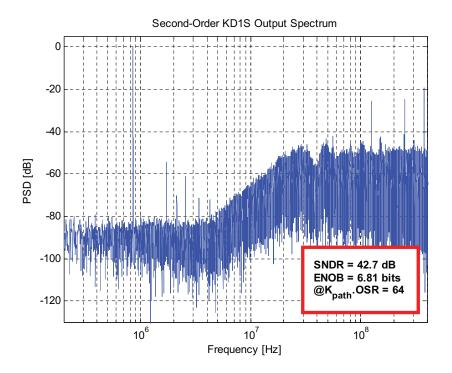
**Figure 7.38:** Measured PSD of the second-order KD1S modulator fabricated in 500nm CMOS. Here,  $f_{in} = 870$  KHz,  $f_s = 100$  MHz,  $f_{s,new} = 800$  MHz,  $K_{path} = 8$ ,  $K_{path} \cdot OSR = 64$ , and BW = 6.25 MHz.
