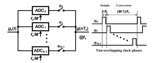
Figure 2.1: Time-interleaved ADCs and the corresponding clock phases.
