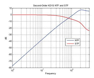
**Figure 5.6:** NTF and STF for the second-order KD1S modulator with  $f_s = 100$  MHz,  $K_{path} = 8$ ,  $f_{s,new} = 800$  MHz,  $f_{un} = \frac{3}{8}f_{s,new} = 300$  MHz, OSR = 8, and  $T_c = 0$ .
