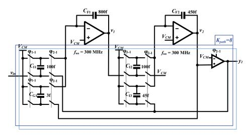
Figure 6.16: A concise representation of the singly-ended, switched-capacitor implementation of the second-order KD1S modulator seen in Fig. 6.15.
