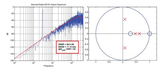
**Figure 5.9:** Matlab simulated PSD of the output and the NTF pole-zero plot for the second-order KD1S modulator with  $f_s = 100$  MHz,  $K_{path} = 8$ ,  $f_{s,new} = 800$  MHz,  $f_{un} = \frac{3}{8}f_{s,new} = 300$  MHz, OSR = 8, BW = 6.25 MHz, and  $T_c = 0$ .
