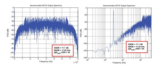
**Figure 5.7:** Spectre behavioral simulation result for the second-order KD1S modulator with ideal components. Here,  $f_s = 100$  MHz,  $K_{path} = 8$ ,  $f_{s,new} = 800$  MHz, OSR = 8, and BW = 6.25 MHz. The quantizer is ideal and has zero delay (i.e.  $T_c = 0$ ).
