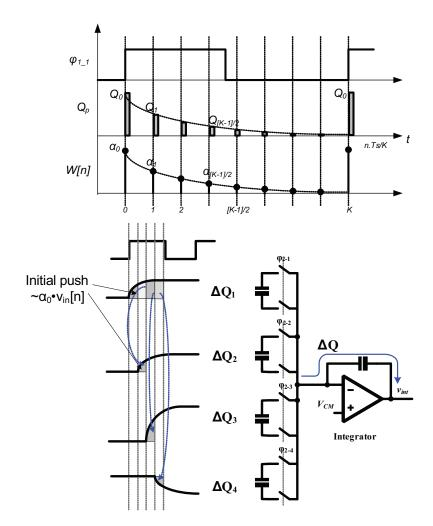
**Figure 4.3:** Illustration of charge-spreading and the equivalent filtering action in a *K*-path SCI.
