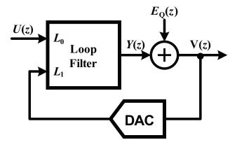
Figure 6.1: A generalized structure of a delta-sigma modulator.
