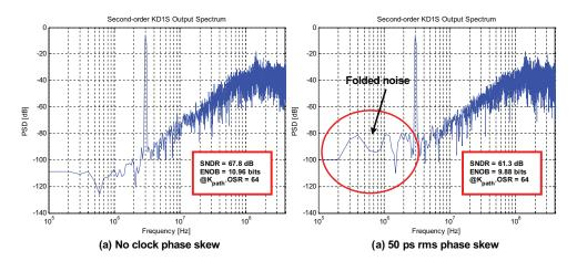
**Figure 5.21:** Spectre simulation showing the noise-folding due to clock-phase skew in the second-order KD1S modulator. (a) Spectrum with no phase skew, (b) spectrum with Gaussian distributed phase skew with 50 ps standard deviation. Here,  $f_s = 100$  MHz,  $K_{path} = 8$ ,  $f_{s,new} = 800$  MHz,  $f_{un} = \frac{3}{8}f_{s,new} = 300$  MHz, OSR = 8, and BW = 6.25 MHz.
