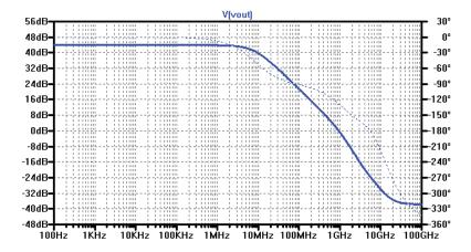
Figure 7.17: Magnitude and phase response of the op-amp seen in Figure 7.16 with 340 fF load. Here,  $A_{OL} = 44$ dB,  $f_{un} = 940$  MHz, and  $PM = 60^{\circ}$ .
