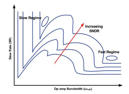
Figure 4.14: Slew-rate vs bandwidth contours for the switched-capacitor integrator.
