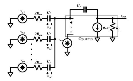
**Figure 4.23:** Equivalent noise schematic during the integration phase with a singlestage op-amp, during the integration phase  $\phi_{2-1}$ .
