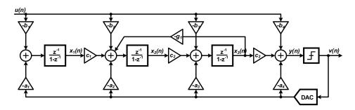
Figure 6.6: CIFB (Cascade of Integrators with Distributed FeedBack) modulator topology.
