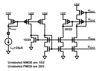
Figure 7.21: Bias generation circuit for the op-amps.
