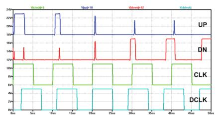
Figure 7.4: Simulation results for the PFD seen in Figure 7.3.
