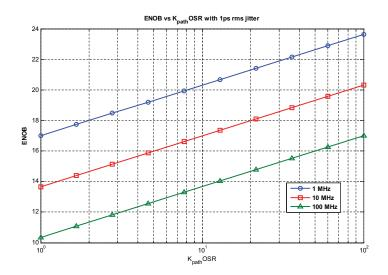
**Figure 4.21:** ENOB vs the effective oversampling ratio for a *K*-path sampling scheme with 1 ps rms clock jitter. The plots are for input frequencies  $(f_{in})$  of 1 MHz, 10 MHz and 100 MHz. The effective sampling frequency for each of the plots is  $f_{s,new} = 2K_{path} \cdot OSR \cdot f_{in}$ .
