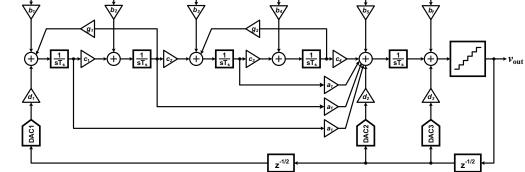
Figure 3.18: The architecture of a wideband continuous-time delta-sigma modulator for wideband data conversion.
