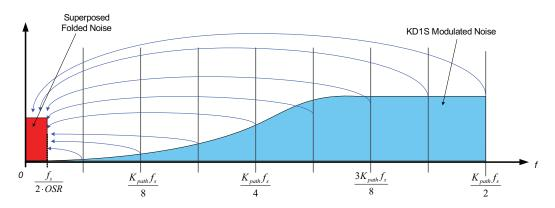
**Figure 4.19:** Noise-folding effects in a KD1S modulator due to path gain mismatches. The shaped quantization noise from the frequencies  $kf_s$ ,  $k = 1, ...K_{path}$  gets folded into the signal band.
