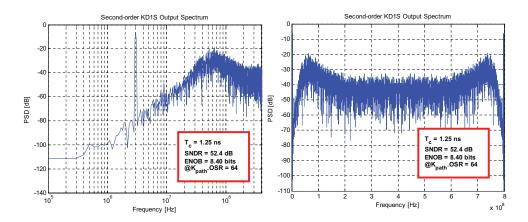
**Figure 5.17:** Spectre simulated PSD (log and linear frequency scales) of the secondorder KD1S modulator with comparator delay  $T_c = 1.25$  ns and the first comparator is clocked on  $\phi_{1-4}$ . Here,  $f_s = 100$  MHz,  $K_{path} = 8$ ,  $f_{s,new} = 800$  MHz,  $f_{un} = \frac{3}{8}f_{s,new} = 300$  MHz, OSR = 8, and BW = 6.25 MHz.
