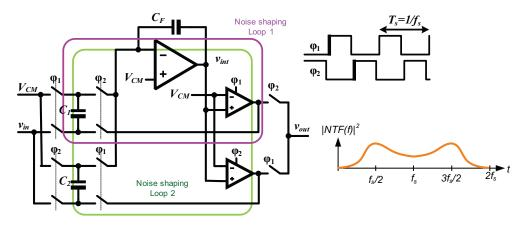
Figure 3.9: A first-order delta-sigma modulator employing double-sampling.
