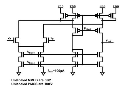
Figure 7.18: Single-ended op-amp employed in the second switched-capacitor integrator.
