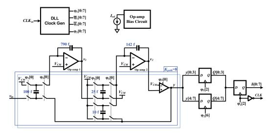
Figure 7.14: A concise schematic representation of the single-ended second-order KD1S modulator with the clock and bias generation circuits.
