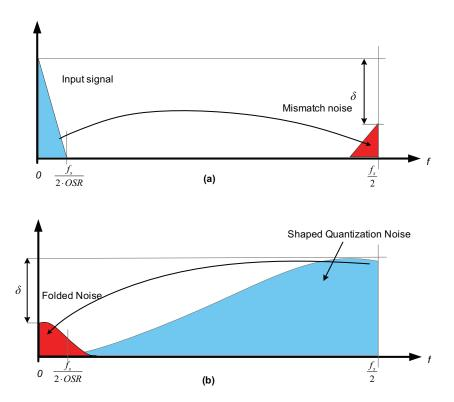
**Figure 3.12:** Noise folding effect due to the path-gain mismatch in a double-sampling DSM. (a) Gain mismatch effect on the input path, (b) Gain mismatch effect on the feedback path where the quantization noise is folded back into the signal band.
