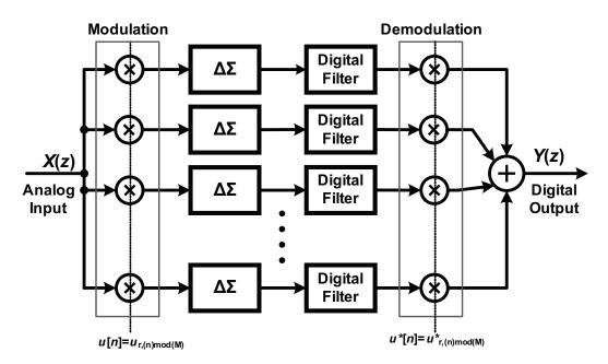
Figure 3.15: A generalized block diagram of the parallel delta-sigma ADC employing modulation.
