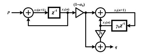
Figure 6.9: A discrete-time linear system representation of the K-path integrator.
