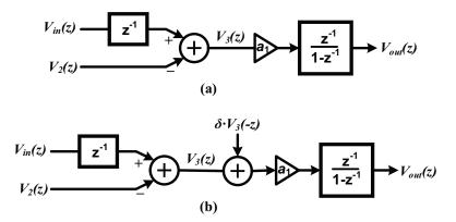
**Figure 3.11:** Signal flow diagram for a double-sampled DSM. (a) case without the path mismatch, and (b) with the folded noise due to the path mismatch.
