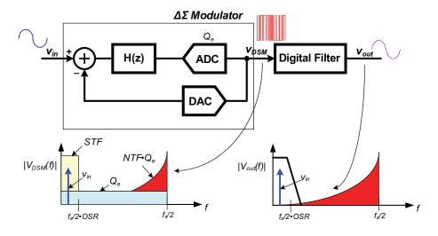
Figure 3.3: Block diagram of an ADC employing Delta Sigma Modulation.
