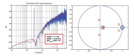
Figure 6.19: Simulated output PSD and the NTF pole-zero plot for the third-order CIFF-type KD1S modulator. Here,  $f_s = 100$  MHz,  $K_{path} = 8$ ,  $f_{s,new} = 800$  MHz, OSR = 8, and BW = 6.25 MHz.
