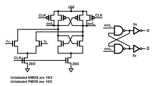
Figure 7.22: The clocked comparator with a static latch.
