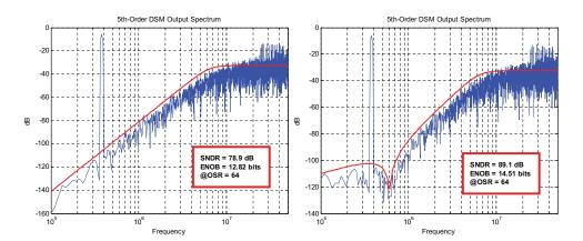
Figure 6.4: Example of NTF zero and pole optimization. Here a third-order single-bit delta-sigma modulator is synthesized for OSR = 64.
