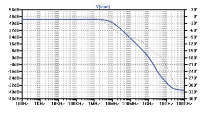
Figure 7.19: Magnitude and phase response of the op-amp seen in Figure 7.16 with 200 fF load. Here,  $A_{OL} = 45$ dB,  $f_{un} = 1.15$  GHz and  $PM = 58^{\circ}$ .
