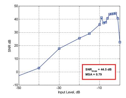
Figure 7.34: Simulated SNR vs input sinewave amplitude for the second-order KD1S modulator.
