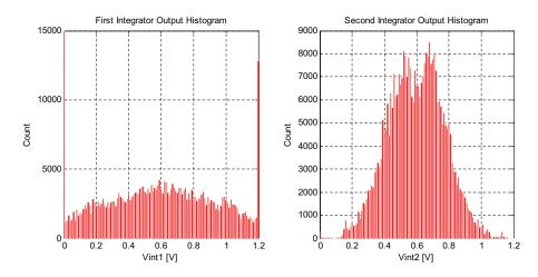
**Figure 5.15:** Histogram of the integrator states for the second-order KD1S modulator for the response seen in Figure 5.14.
