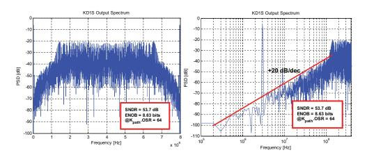
**Figure 4.8:** Simulation results (PSD of the output with linear and log frequency axes) for a KD1S modulator with ideal components. Here,  $f_s = 100$  MHz,  $K_{path} = 8$ ,  $f_{s,new} = 800$  MHz, OSR = 8, and BW = 6.25 MHz.
