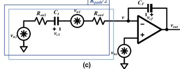
Figure 4.22: Noise analysis for the *K*-path integrator: (a) Equivalent noise during the sampling phase for each of the capacitors. (b) Equivalent noise schematic for (a). (c) Equivalent noise schematic during the integration phase.
