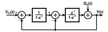
Figure 3.6: A discrete-time second-order DSM.
