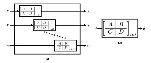
**Figure 6.10:** Illustration of the generalized ABCD matrix for a set of M integrators, (a) individual ABCD matrices for the integrators with individual inputs and outputs, (b) combined ABCD matrix for all the integrators.
