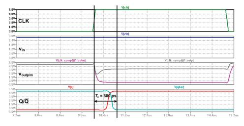
Figure 7.23: Transient simulation of the clock comparator seen in Figure 7.22.
