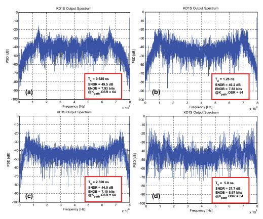
Figure 4.16: Effects of comparator delay on the SNR of a first-order KD1S modulator simulated in Spectre with  $f_s = 100$  MHz,  $f_{un} = 300$  MHz,  $K_{path} = 8$ , OSR = 8, and BW = 6.25 MHz. The KD1S modulators were simulated with a respective clocking scheme to minimize the loop-delay. (a)  $T_c = 625$  ps, (b)  $T_c = 1.25$  ns, (c)  $T_c = 2.5$  ns, and (d)  $T_c = 5.0$  ns.
