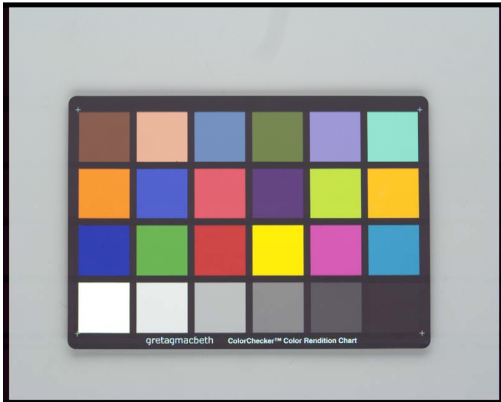
Figure 5.27 Low conversion gain image taken under 1000 Lux illumination with 30FPS
