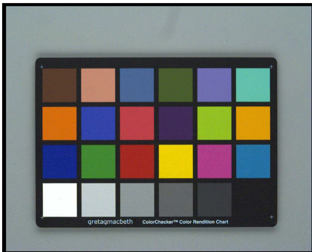
Figure 5.29: High conversion gain image taken under 10 Lux illumination with 5FPS
