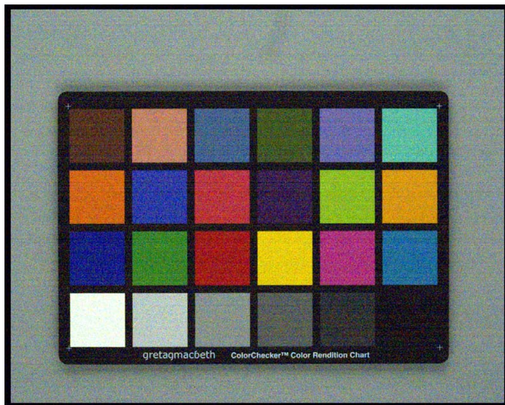
Figure 5.31: Image taken under 1 Lux illumination and 200ms integration time at high conversion gain mode with 5FPS
