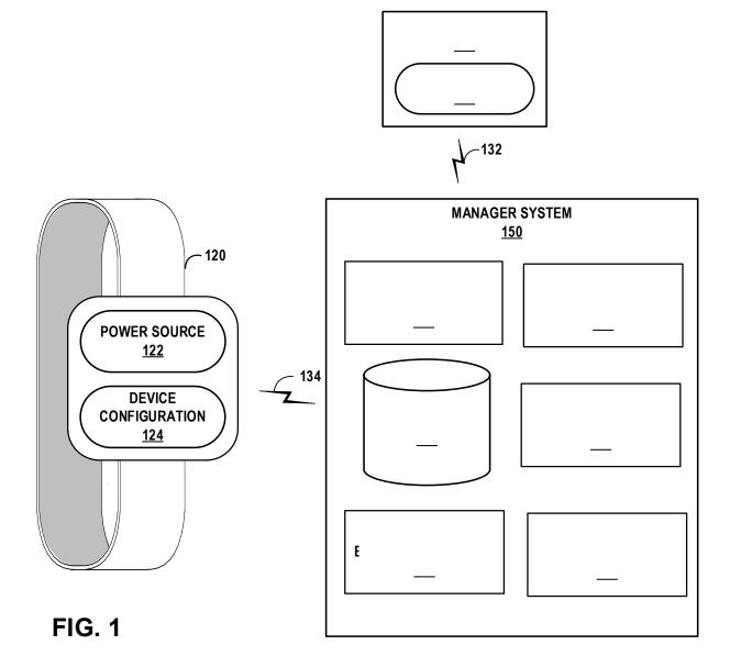
Manager system 150 may be communicatively coupled to computing devices 100 via connection 132, as well as communicatively coupled to wearable computing device 120 via connection 134. Connections 132, 134 may include wired or wireless connections and may be direct or require one or more intermedia network devices and may or may not traverse the Internet. Examples of connections 132, 134 include near-field communication (NFC),
