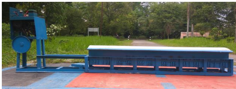
Figure 1 Power generation equipment using a speed bump [6]
