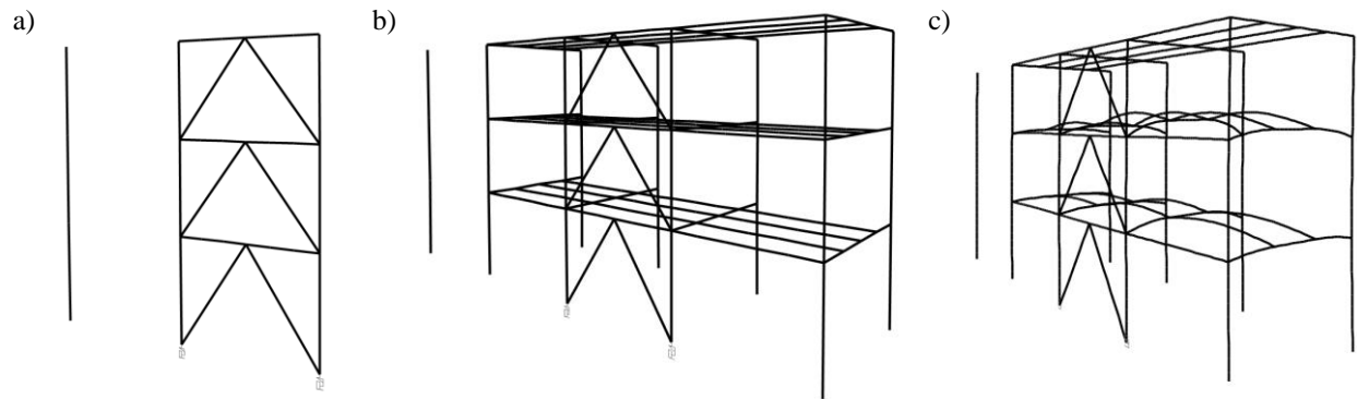
Figure 4: Numerical models: a) 2D Model P; 3D Model M; and c) Floor beam vibration mode (from Model M).
