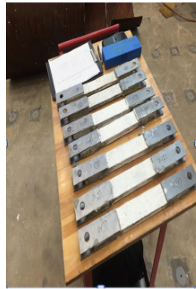
(c) Coupons after gluing steel
