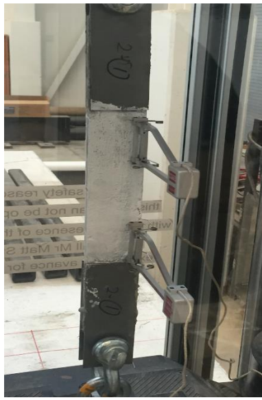
(b) Initial clevis test set-up with two clip-on extensometer
