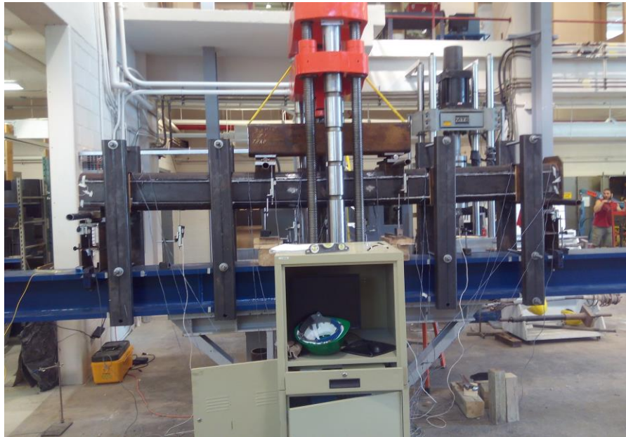
Figure 2: Flexural bending experimental test set-up
