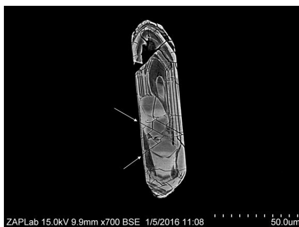
Figure 2-2: Shocked zircon F397 from V15-55, showing two orientations of planar fractures (white arrows) and some more typical irregular cracking due to differential expansion due to metamictization.
