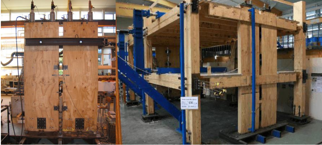
Figure 4: Coupled walls and two-storied building model
