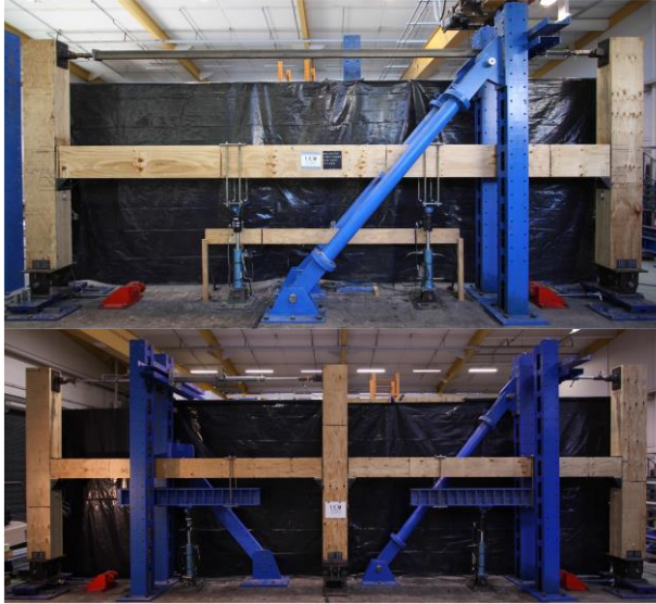
Figure 18: Gravity frame test structures and details including draped tendon layouts
