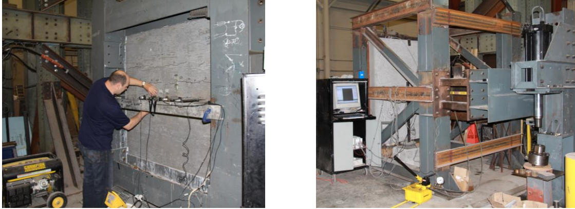
Figure 2: Test Setup: (a) Testing Frame Front View; (b) Data Acquisition System and Testing Frame Layout
