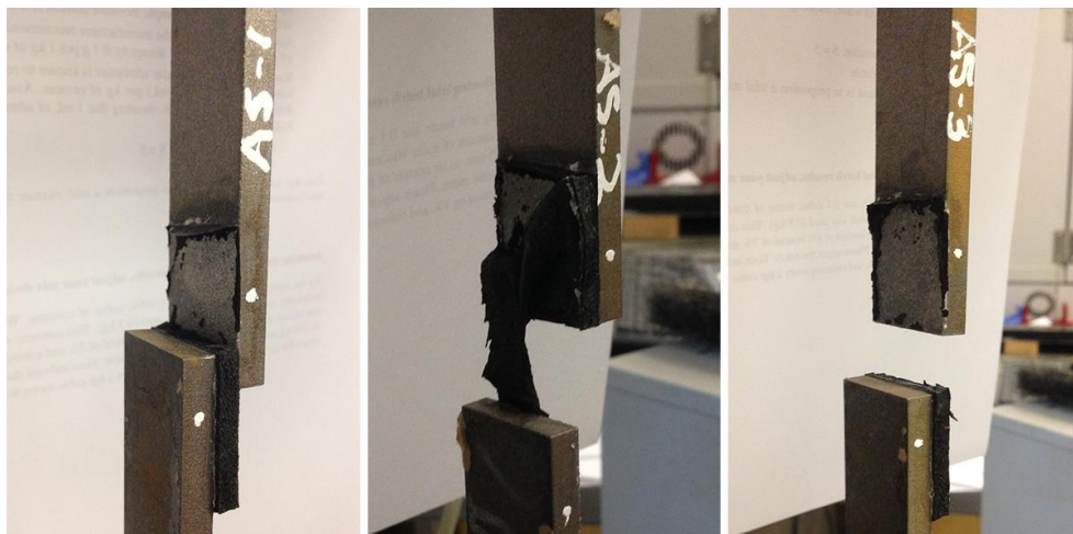
Figure 9: Damage scenarios in adhesive shear strength tests
