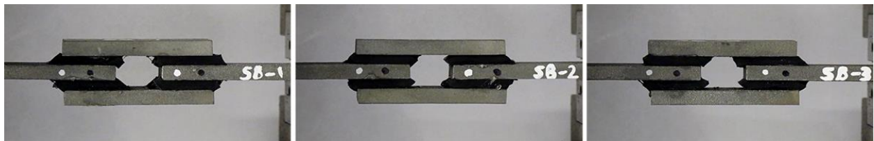
Figure 5: Initiation of de-bonding in shear bond tests
