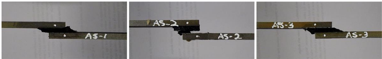
Figure 8: Initiation of de-bonding in adhesive shear strength tests
