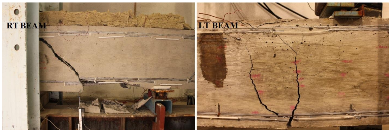
Figure 2: The tested beams after fatigue failure – shear failure at room temperature (left) and flexural failure by reinforcement rupture at low temperature (right)
