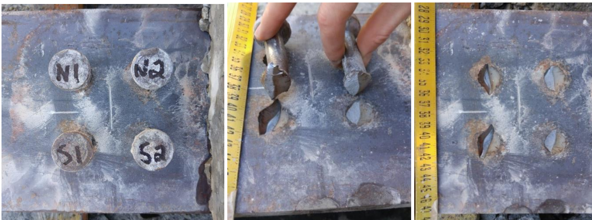
Figure 5: Critical Stud Group in Autopsy of Specimen S3
