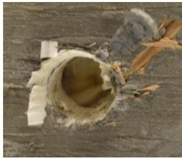
(a.2) Shearing of ribs (a) Ribbed-surface bars
