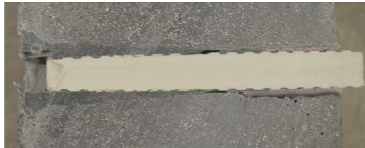
(b.2) Bar slippage from the headed anchor (b) Headed-end bars
