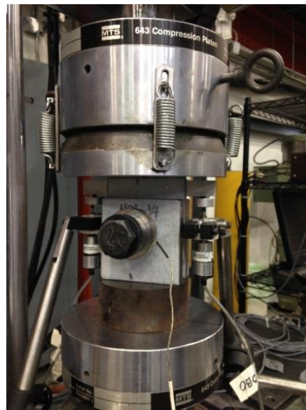
Figure 5: Compression slip test setup
