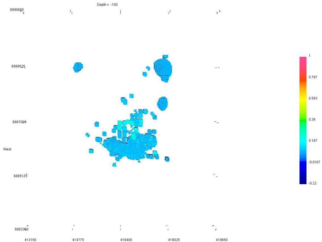
Figure 3.12: A density isosurface of the shallow, high density anomaly. The figure displays densities greater than +0.1 \text{ g/cm}^3 within the top 400 metres. Units on the right side represent density in \text{g/cm}^3 above or below 2.67 \text{ g/cm}^3 .
