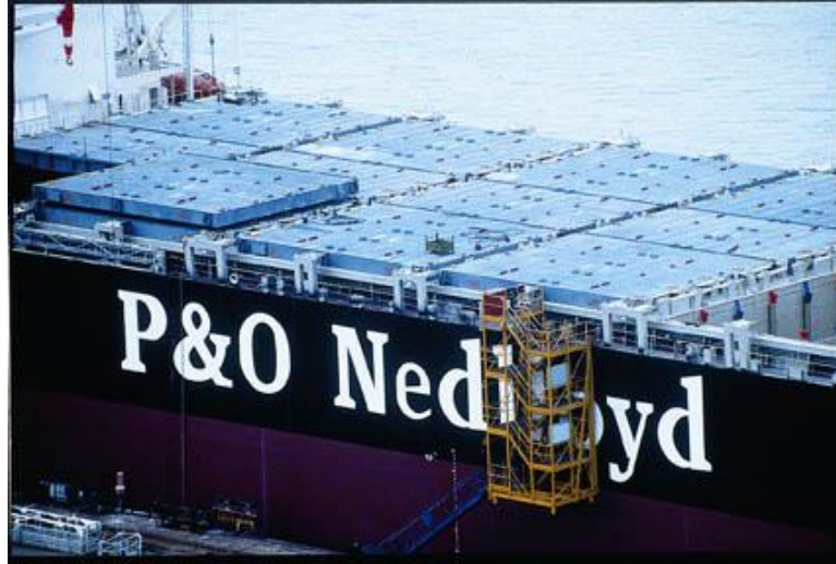
Figure 20: Container ship with lift off/lift on hatch covers (© TTS Group ASA)
