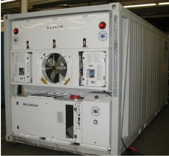
Figure 6: Refrigerated container showing refrigeration unit (© 2009 Sarah Klunge)
