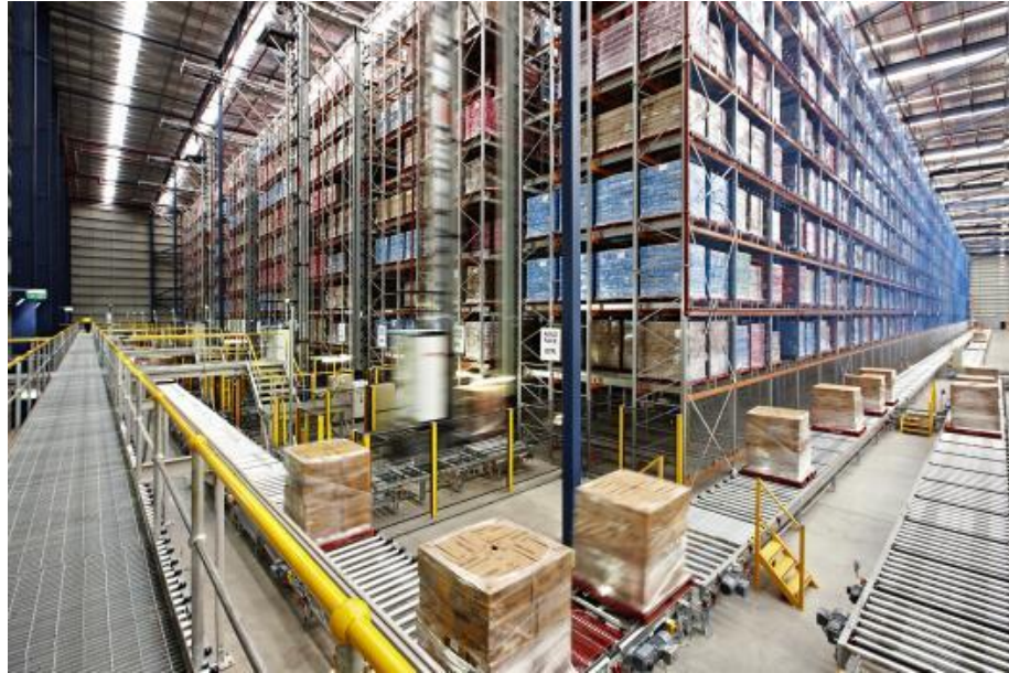
Figure 26: Example of pallet high rise racking automated storage and retrieval system (© Dexion China)
