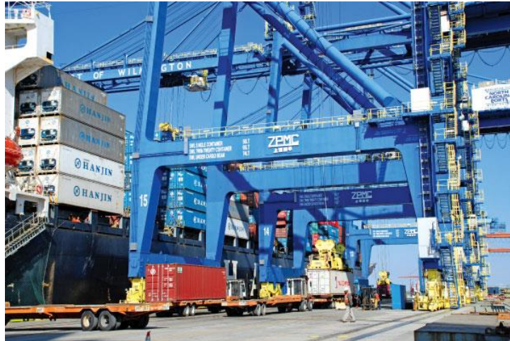
Figure 12: Rail-mounted cranes stacking containers on truck chassis (Source: O’Reilly 2011)
