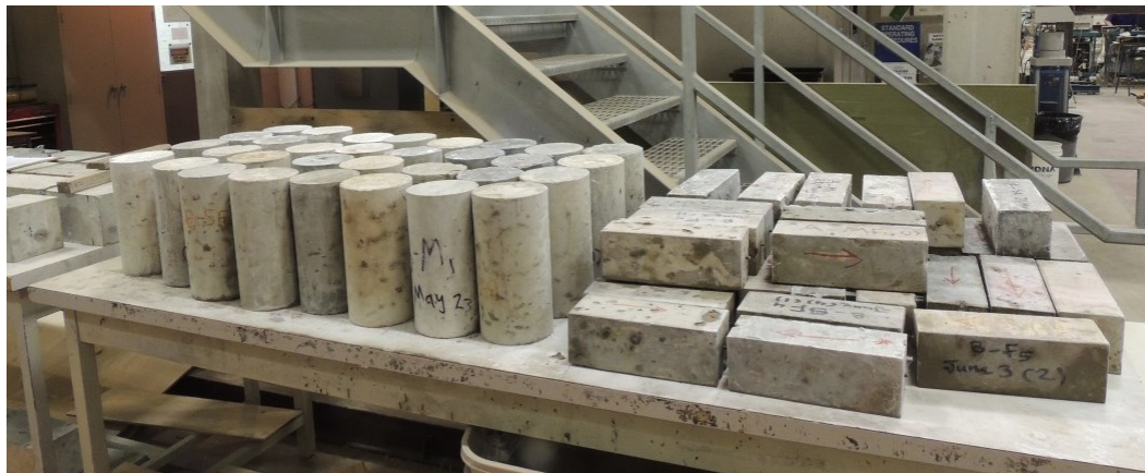
Figure 6.1 – TSC specimens before the exposure to chemical sulfate attack.
