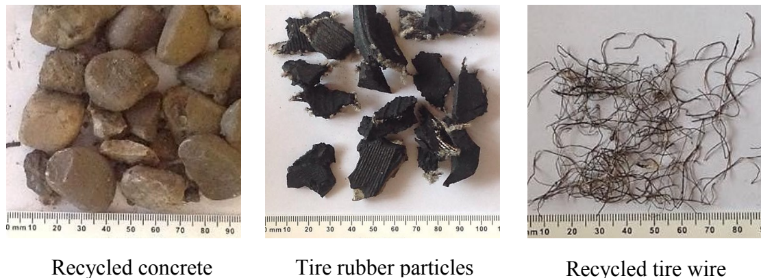
Figure 7.1 – Illustration of ingredients used in producing various TSC mixtures.
