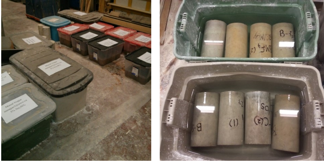
Figure 6.2 – TSC specimens are fully immersed into tanks filled with a solution of 5% sodium sulfate (chemical sulfate exposure).
