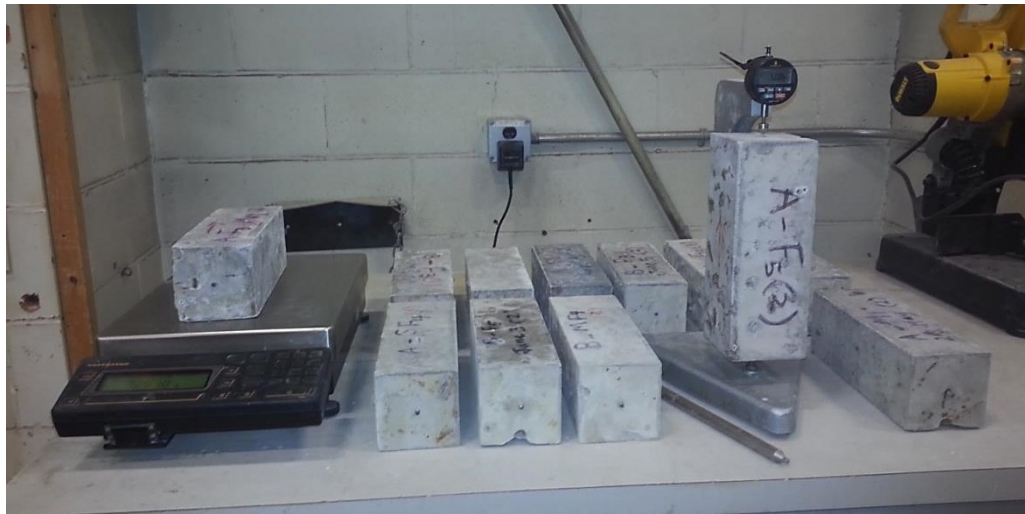
Figure 6.3 – Determining the change of mass and length for TSC specimens after chemical sulfate attack.
