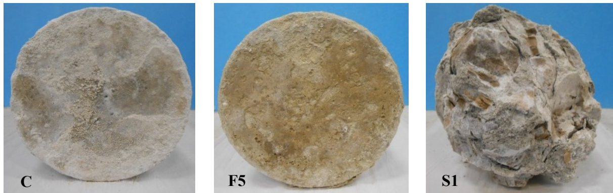
Figure 6.15 – Comparison between bottom surface of C, F5 and S1 specimens after 6 months of physical sodium sulfate exposure.
