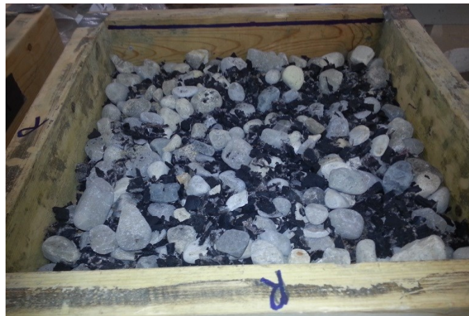
Figure 7.2 – Preplacing recycled materials to produce sustainable TSC.
