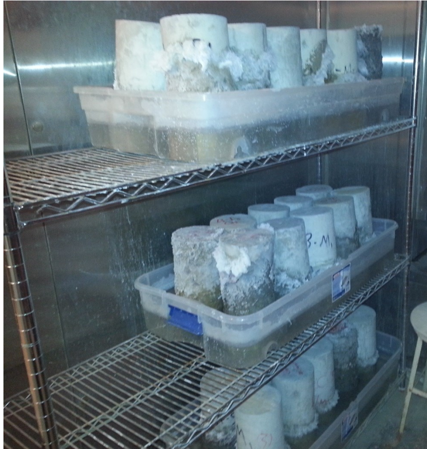
Figure 6.4 – TSC specimens are partially immersed in a solution of 5% sodium sulfate inside an environmental (physical sulfate exposure).
