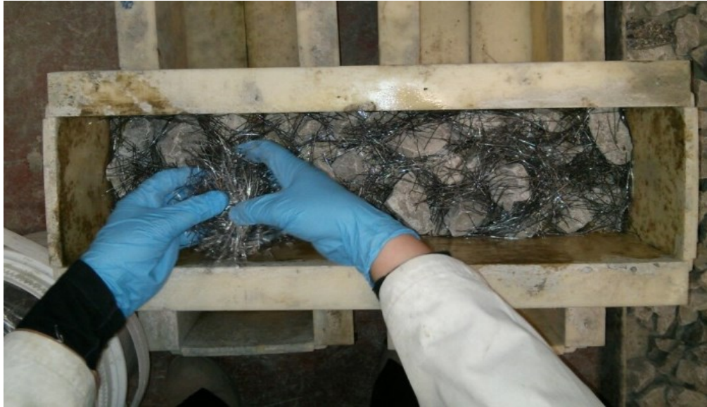
Figure 5.1 – Preplacing coarse aggregates and steel fibres.
