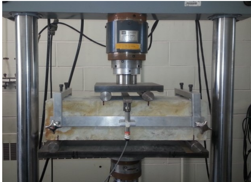
Figure 5.2 – Flexure test setup.
