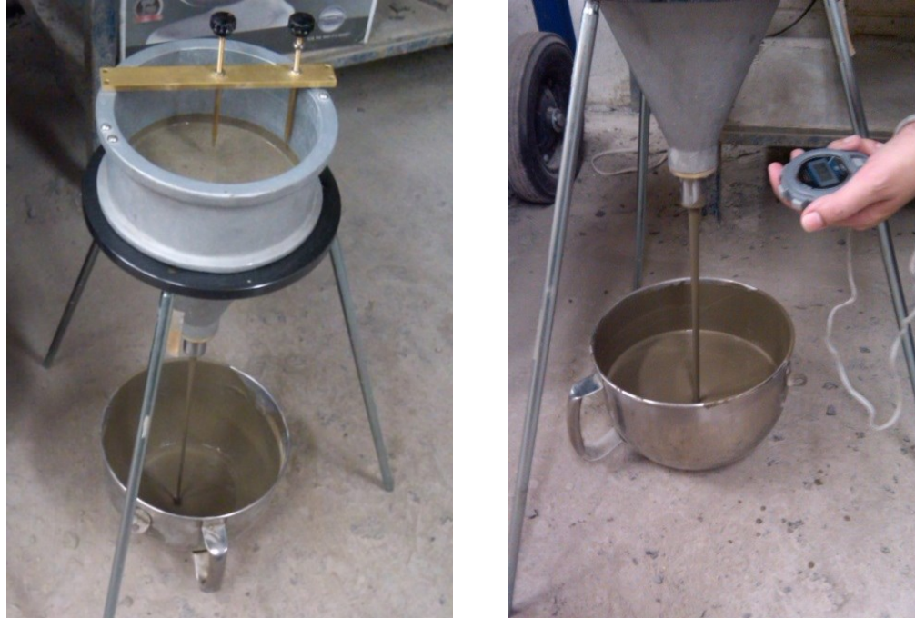
Figure 3.2 – Flow cone test.
