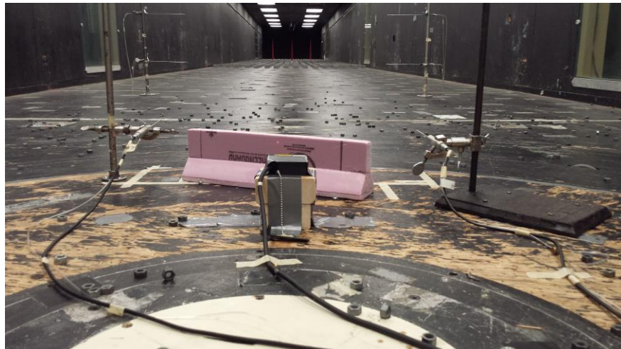
Figure 3: View of the model and wind tunnel setup for one of the trials
