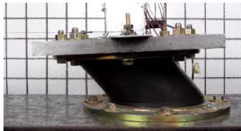
Figure 7: Large positive rotation of the bearing in the HSS64x64x4.8 subassembly resulting in single curvature
