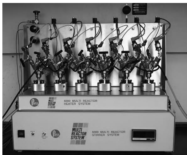
Figure 4.5 Multiple slurry reactor used for the hydrogenolysis of glycerol 35 (adopted with copyright permission)
