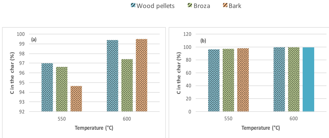
Figure 4.9. Carbon Contained in Char Following Gasification at 550°C and 600°C under: (a) A CO 2 -water atmosphere and (b) A He-water atmosphere. Data reported is the average of at least 15 repeats with a +/- 3-6% standard deviation.
