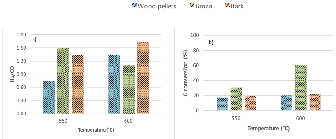
Figure 4.8. Changes of (a) H 2 /CO ratio and (b) Conversion of Biomass Contained Carbon (CBCC) into synthesis gas with temperature; during steam gasification of wood pellets, broza and bark, under a CO 2 atmosphere; for 40 min reaction time. Data reported is the average of at least 15 repeats with a +/- 3-6% standard deviation.
