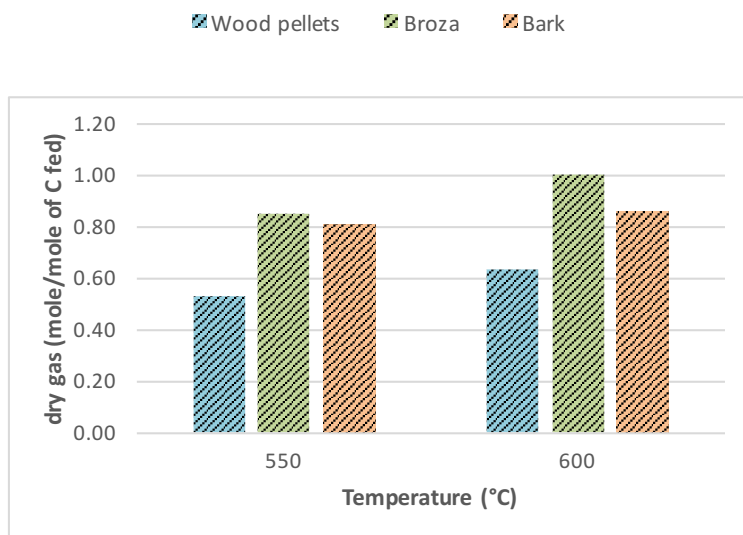
Figure 4.2. Changes of dry gas yields with temperature for steam-helium gasification of wood pellets, bark and broza. Gasifying agents: He at 1. atm and H 2 O at 0.5 atm. Data reported is the average of at least 15 repeats with a +/- 3-6% standard deviation.
